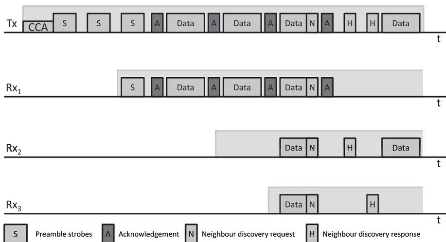
Fig. 2. Mobility mode for data transmission in MA-MAC.
