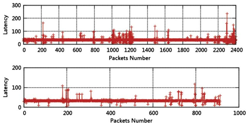
Fig. 11. Latency (in ms) in packet delivery for a handover threshold= -30 dB m. Above: slow movement (app. 0.5 m/s). Below: fast movement (app. 1.5 m/s).
