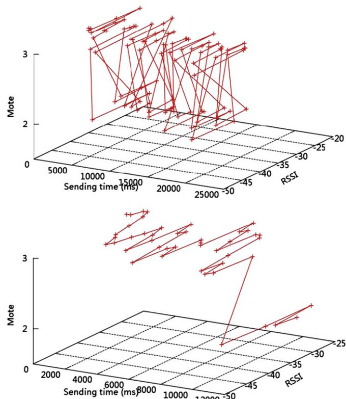
Fig. 7. Handover without the oscillation avoidance mechanism implemented (top) and when the oscillation avoidance mechanism was implemented (bottom).
