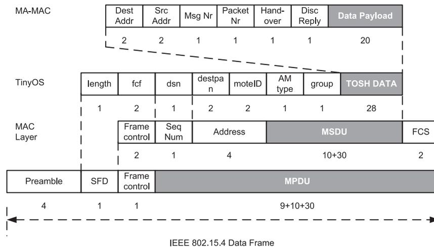
Fig. 5. Placement of the MA-MAC header in the TinyOS radio stack.
