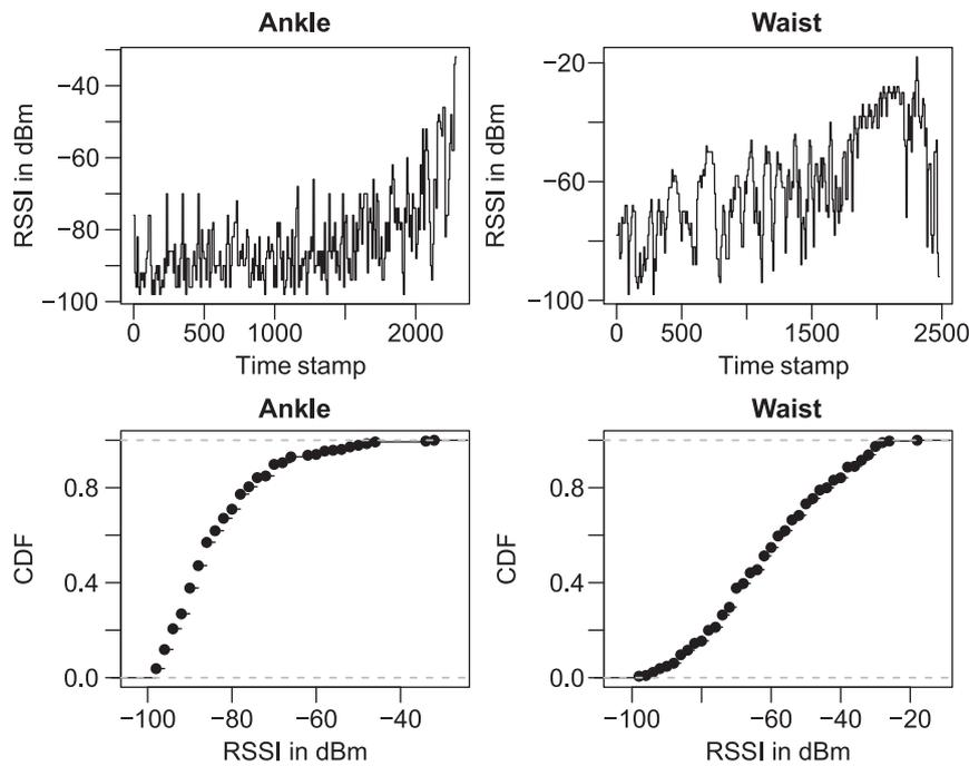
Fig. 4. The impact of position on the fluctuations of the RSSI values obtained from acknowledgement packets during mobility. The figures above display the raw measurements while the ones below display the cumulative distribution functions (CDF) of the raw measurements.
