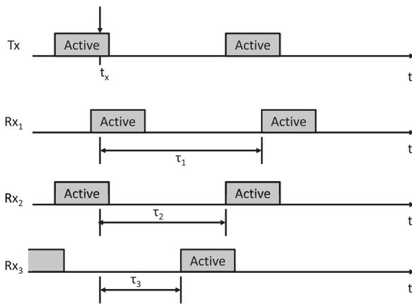
Fig. 1. The delay in packet transmission when a communication link is broken amidst transmission.
