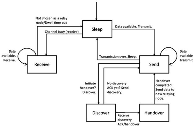
Fig. 3. The finite state machine of MA-MAC.
