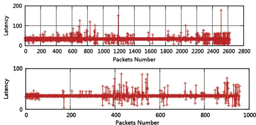
Fig. 12. Latency (in ms) in packet delivery for a handover threshold =  $-40$  dB m. Above: slow movement (app. 0.5 m/s). Below: fast movement (app. 1.5 m/s).
