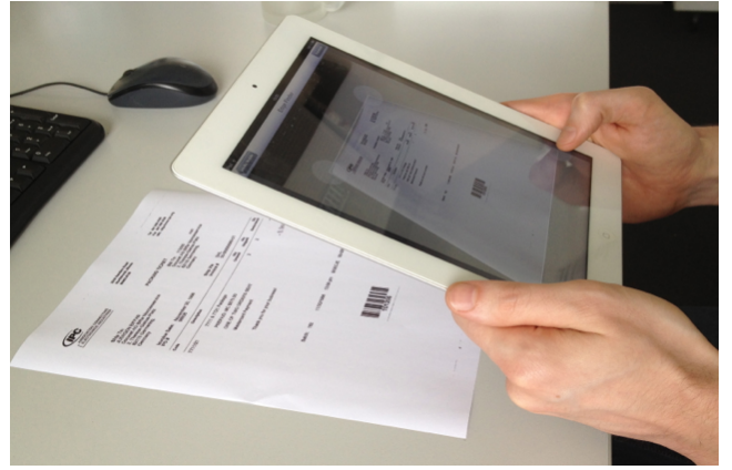
Figure 1: Capturing a business document with our iOS application. The current view shows the Intellix edge detection algorithm.
