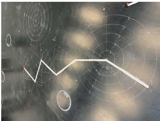
Fig. 7. The trajectory for a mobile robot in a polar coordinate system for self-navigation.
