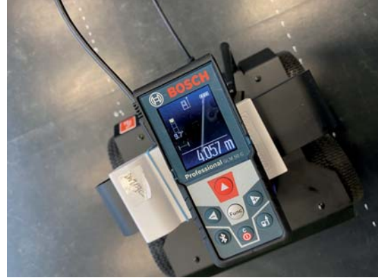
Fig. 1. Using a laser-based distance sensor as a reference to determine measurement statistics
