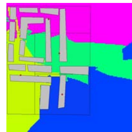
Fig.5. CANDY: 802.16 WiMAX BS constellation and RF coverage via COST WI
