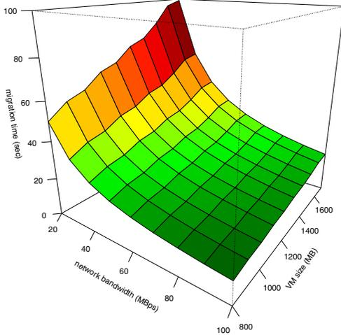
Fig. 4. Average migration time for virtual machines of size between 800 MB and 1700 MB and network bandwidth between 20 MBps and 100 MBps.
