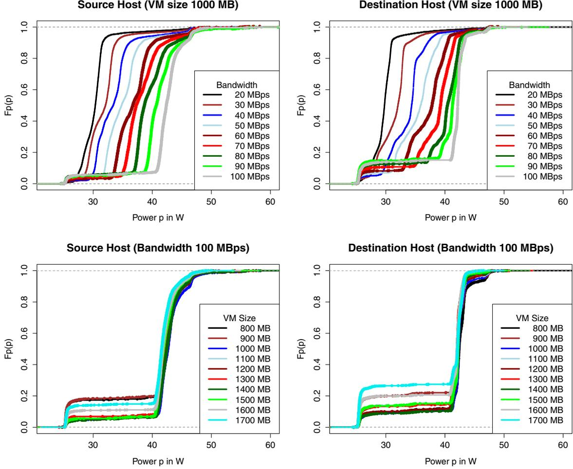
Fig. 3. The distribution function  $F_P(p)$  of the power consumption of the source and the destination server during a migration. Top: When the VM size was 1000 MB. Bottom: When the network bandwidth was 100 MBps.
