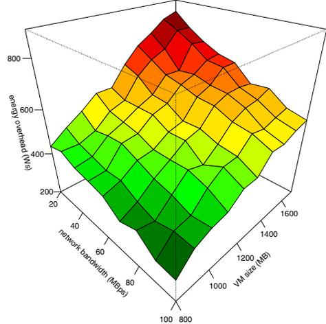
Fig. 5. Average energy overhead during migration of virtual machines of size between 800 MB and 1700 MB and network bandwidth between 20 MBps and 100 MBps.
