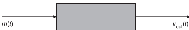
Figure 11.1 The accuracy of a sensor is usually determined in a lab setting by exposing the sensor to a measurand of known values (which can be measured by a standard device) and by comparing its response to reference values.
