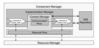
Figure 1: Conceptual COMQUAD container architecture [5]
