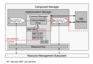
Figure 2: Detailed COMQUAD container architecture
