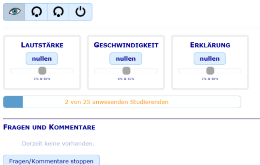
Figure 5.6.3: Tutor view of RNUW's ARS tool. Design of boxes as in Figure 5.6.2. Icons on top (left to right): pause ARS (retaining all votes), reset ARS, reset Q&A, disable ARS and Q&A. Bar below boxes: number of attendees logged-in into platform. Area below: tutor view of Q&A tool (button far bottom: pause Q&A tool retaining all contributions).
