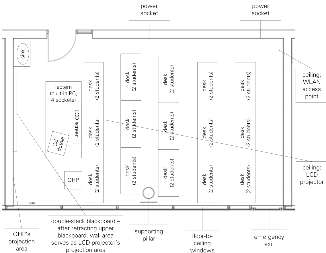
Figure A.0.1: Example of a modern lecture room layout. Parallel utilisation of OHP and blackboard or LCD projector is possible. The tutor can utilise the computer in the lectern, or bring their own laptop computer, or even use both to separate presentation and feedback.
