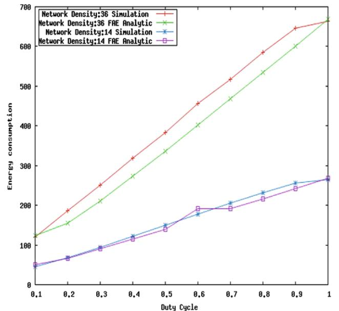
**Fig. 5** Energy consumption as duty cycle changes
