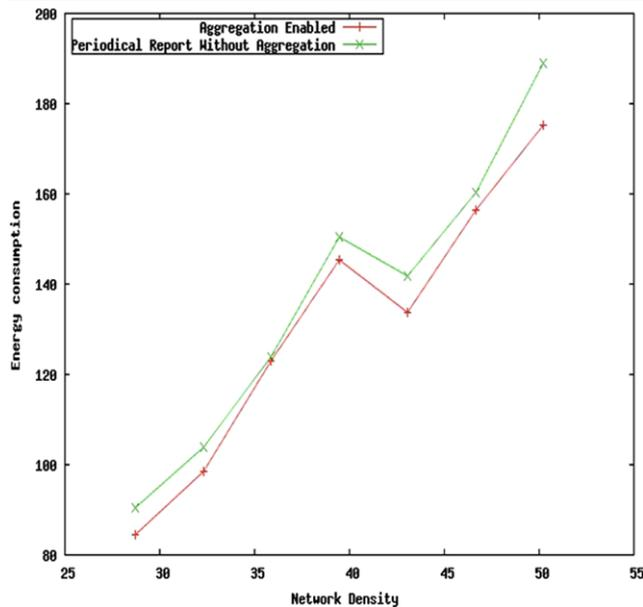
**Fig. 8** Data aggregation impact on energy consumption
