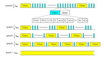
Fig. 2. Synchronization frequency adjustment in MS-MAC
