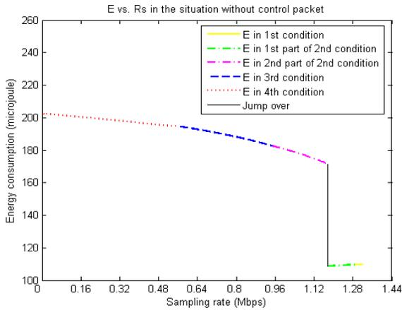
Fig. 6. Relationship between the extra energy cost and the sampling rate in the situation without control packets
