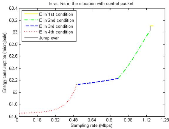
Fig. 5. Relationship between the extra energy cost and the sampling rate in the situation with control packets
