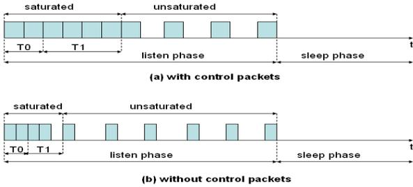
Fig. 3.  $T_1$  for different scenarios
