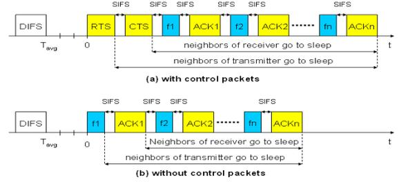
Fig. 2. Sleeping durations with and without control packets
