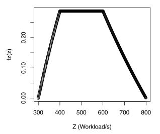
Fig. 2. The pdf of Z (workload per second) when both the arrival rate (number of requests per second) and the workload size (in MB) are uniformly distributed: the first, U(10,20) and the second, U(30,40).
