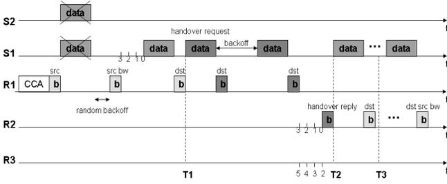
Fig. 2. Working principle of the handover mechanism
