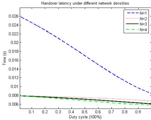
Fig. 3. Overall handover latency under different network densities
