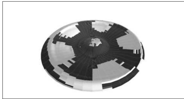
Figure 5.9: Phase pattern of the out-of-phase vibration component at 580 Hz.
