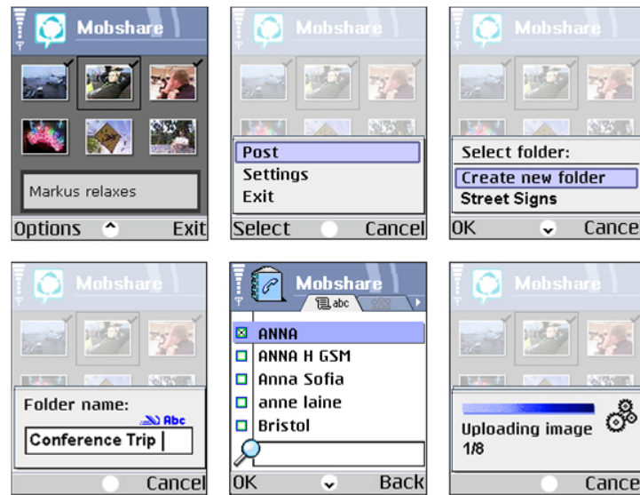
Figure 3.4.: The posting process where (a) the images are selected, (b) posting initiated, (c) new folder created, (d) named, (e) the people selected, and (f) finally the images are uploaded. [SVPN04]
